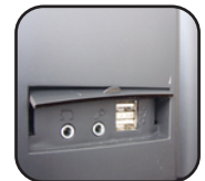
Easy access front I/O (USB 2.0 x 2, Speaker / Mic ports)
