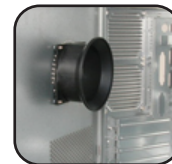
CPU air guide & VGA card venting hole
