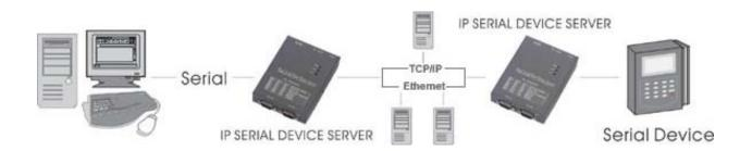
» Easy installation / IP to Serial Device Server / Paired Mode«
