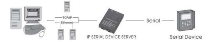
» Easy installation / IP to Serial Device Server / Direct IP Mode / Virtual COM Mode
