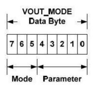
If a device accepts the VOUT\_MODE command, the Mode and Parameter are retained until changed with another VOUT\_MODE command or until the bias power is removed.
